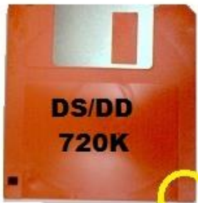
DS/DD "Double Density" "Low Density" 720K No hole at bottom right
