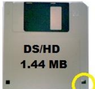
DS/HD "High Density" 1.44 MB Note hole at bottom right
