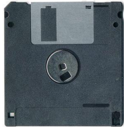
DS/HD "High Density" 1.44 MB Note hole at bottom right
